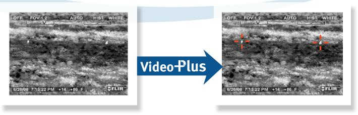
Video is processed and icon overlays (red crosshairs) indicate moving target detections.
