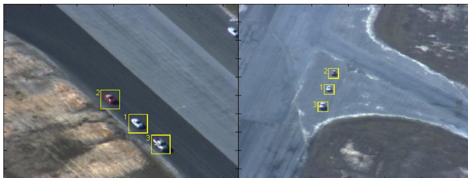
Figure 10: Substantial change in scale occurs during the 43 sec.-duration EgTest02 video. The change in scale is tracked by estimating the target bounding box sizes from the areas of the segmented target blobs.
