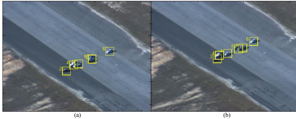
Figure 13: In the EgTest02 video, two sets of three vehicles pass each other with very little separation, but are tracked effectively via a combination of motion- and feature-based measurements with JPDA.
