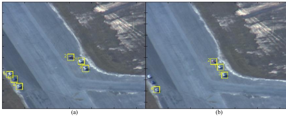
Figure 11: Rapid camera panning between frames (a) and (b) causes three targets to exit and then reenter the field of view. Tracks are dropped when targets exit the field of view and are reinitialized when targets reenter. Rapid camera panning is effectively accounted for via frame registration.
