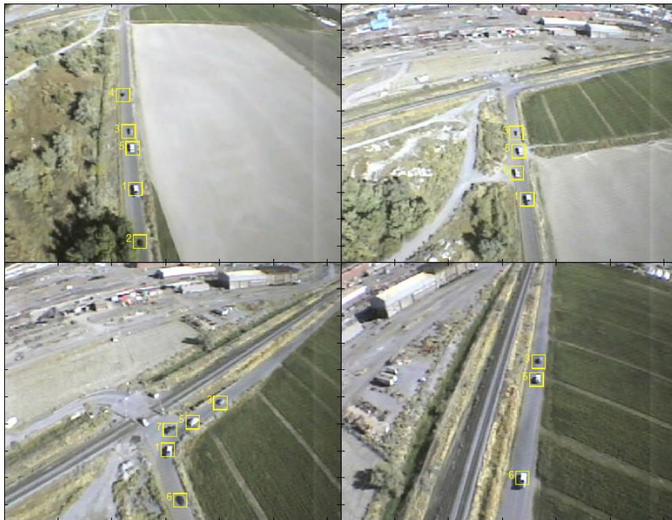
Figure 2: Screenshots from the image plane tracker display for the Procerus™ Convoy Following Zagi flight.
