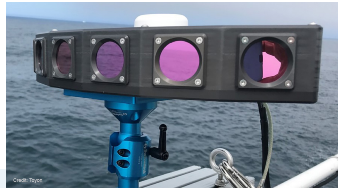
Six LWIR camera sensors provide a wide field of view.
