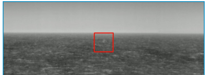
Screen shot of Marine Observer software. Red box indicates an automatically detected whale blow.
